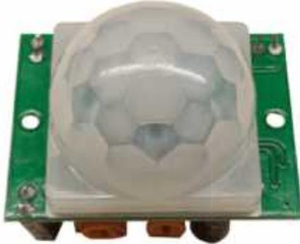
Gambar 3. Sensor PIR (Tampak Atas)
