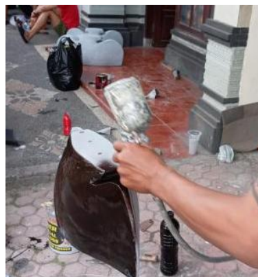
Fig. 4. Base coating process with spraying
