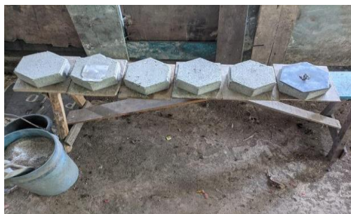
Fig. 4. Product results from paving blocks from waste glass
