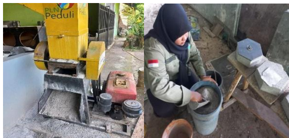
Fig. 3. Manufacturing of paving block products from waste glass
