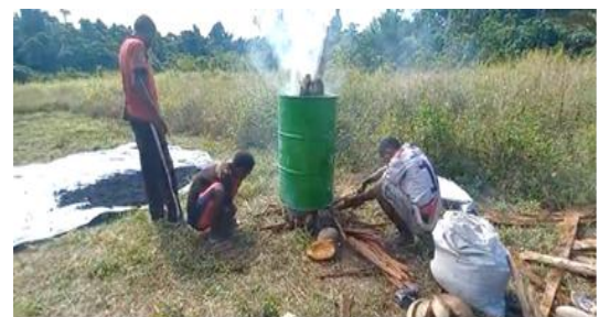
Fig. 7. Carbonization of palm oil mill residue and sago pulp waste
