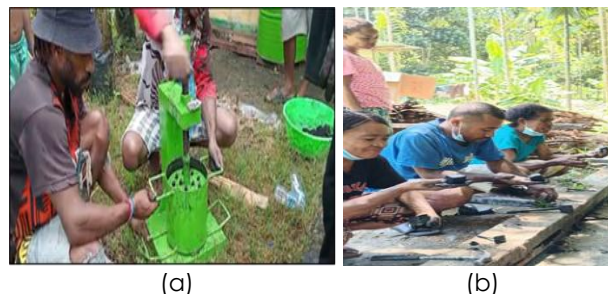
Fig.12. Briquette molding, (a). Tube-shaped briquette, (b). Box-shaped briquette
