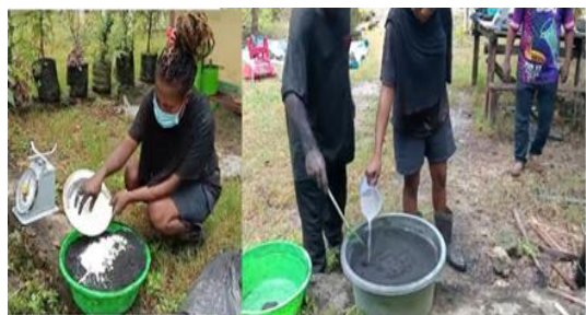
Fig. 10. Mixing charcoal, tapioca (binder), and hot water
