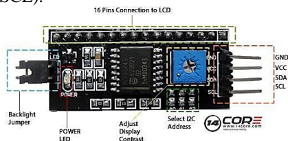
Sumber : https://www.14core.com/wiring-i2c-module-on-16x2-lcd-with-scl-sda/ Gambar 10. Modul I2C LCD Beserta Penjelasannya
