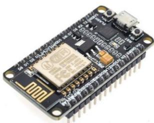
Gambar 4. NodeMCU ESP8266
