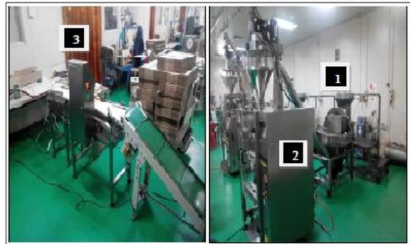
**Fig. 1.** Nitrogen packing process machines (1 is sieving machine, 2 is auger filler machine and three is weighing machine)
