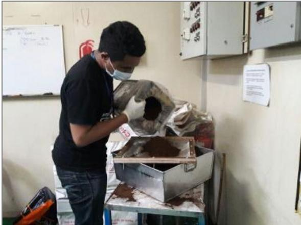
**Fig. 12.** Sieving of coffee powder to smaller and consistent size
