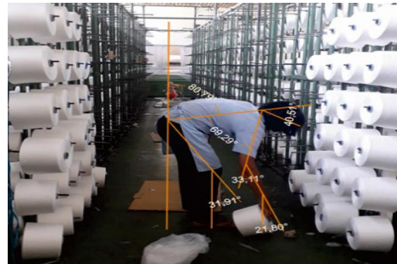
Fig. 3. Withdrawal of work element angle
