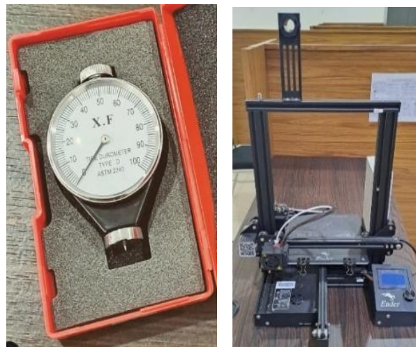
Fig. 3. Durometer shore test (a) and FDM 3D Printer (b)
